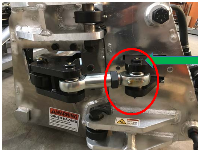
Figure 9: Method 2 – Fold Cylinder Adjustment Method 2 - Double Heim Joint
